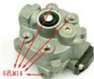
5400-4564114 继动阀(RL3518LE-A) relay valve
