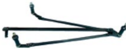
5320-6211511 雨刮支架 (三刮) wiper bracket
