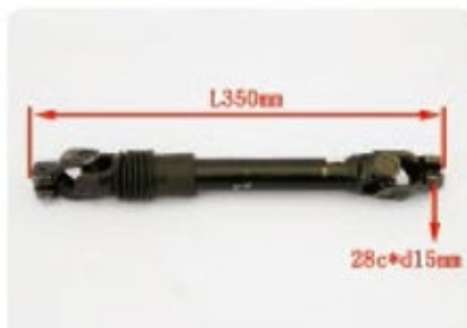
5007-4432611 方向机万向节及伸缩叉总成 U-joint and flex fork assy, transversor
